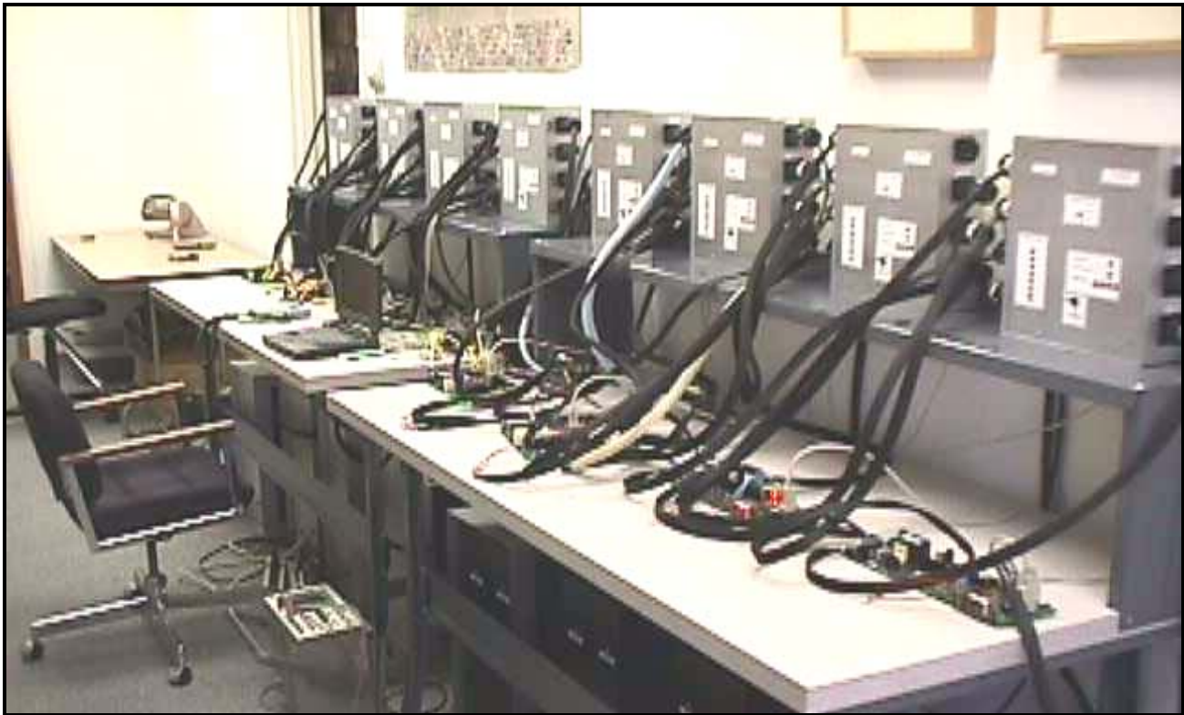
Test bench for custom industrial controllers designed and manufactured for a Silicon Engines customer. Each unit is given complete continuous functional test under load before being shipped under warranty.
